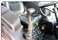
The Front loader SCV is on the front right side of the tractor and the Joy stick is located on the right fender which makes operating the front loader much more convenient.
