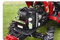
3 cylinder diesel engine is in compliance with the EPA emission standards with the record of over 1,500hrs of IPA hurdle test
