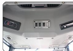
The wind outlet of the heater and air conditioner are concentrated to the operator maximizing the performance.
