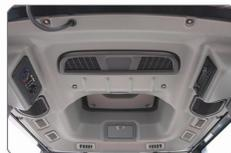
The wind outlet of the heater and air conditioner are concentrated to the operator maximizing the performance.
