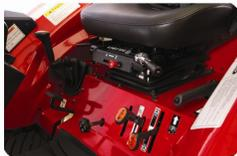
The differential lock improves traction on slippery surface.
